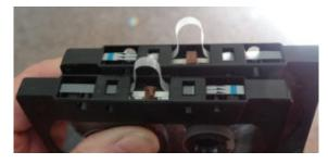
The pressure pad in the upper cassette is fine, but little is left of the pad in the lower one, thanks to M.O.T.H.S....
